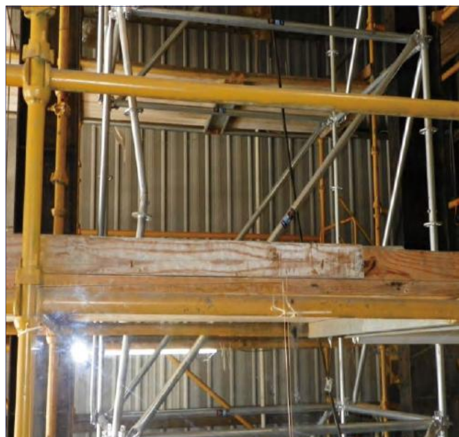
Typical deflection of leg at failure
